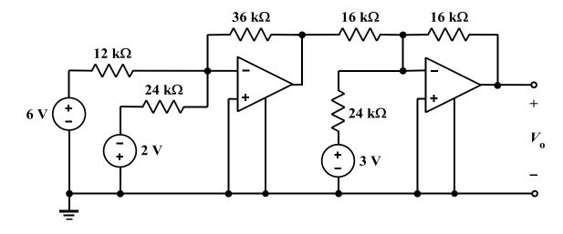
Assume the op amps are ideal, and determine the output voltage,  $V_o$ .
